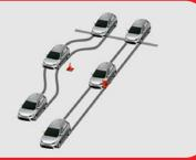
Antilock Brake system: With electronic Brake-force Distribution helps maintain vehicle stability and driver control when braking. It includes a Brake Assist function that increases the braking force when the brakes are suddenly applied to make an emergency stop.
