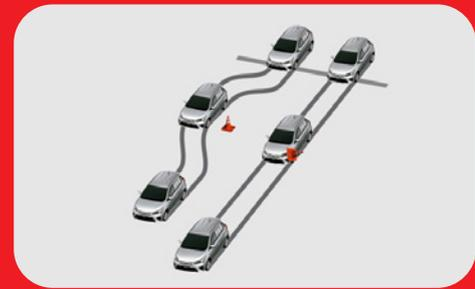
**Antilock Brake system:** With electronic Brake-force Distribution helps maintain vehicle stability and driver control when braking. It includes a Brake Assist function that increases the braking force when the brakes are suddenly applied to make an emergency stop.
