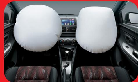
**SRS Airbags:** Are adapted for the driver's and front passenger's seats. In addition, the body structure efficiency absorbs and distributes energy from frontal and side impacts, helping reduce cabin deformation.
